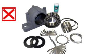
Standard assemblies require precision assembly techniques including using feeler gauges to set the correct bearing radial internal clearance for optimum life. Difficult to do in the field and the high risk of contamination in harsh environments.
